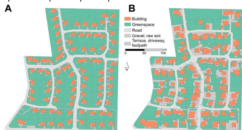
Fig. 3: Draft in the development plan (A) and actual implementation digitized from May 2016 orthophotos (B).
